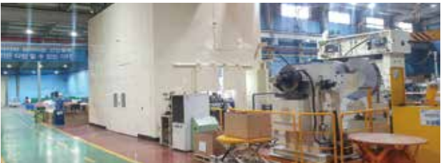
Soundproof booth installed to prevent hearing impairment
