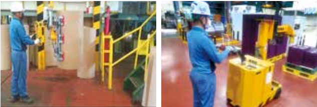
Dedicated paper pipe insertion device
